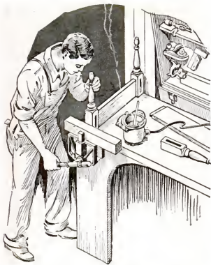
Clamping work between the vise and a solid backing of "four by fours." Right, view showing end of cabinets and angle brace under the bench top
